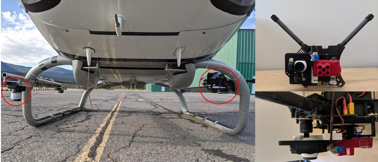
Figure 2. Left image shows that two RGB cameras were mounted on the right skid step and the drone cameras are mounted on the left. Right images show engineering that was done on the drone mount and cameras to collect images on a helicopter.
