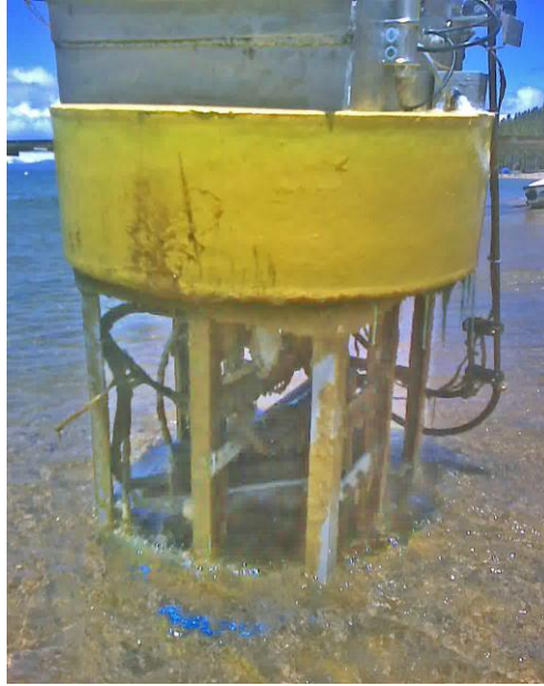
Figure 12. The buoy upon removal on June 2, 2011 showing the amount of algae growth on the aluminum infrastructure. Upright, at the right side of the photo, are the internal sample intake lines, which would hang down in to the water column during normal operation.
