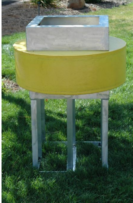
Figure 1. Structural portion of the buoy without sensors or sensor mounts.
