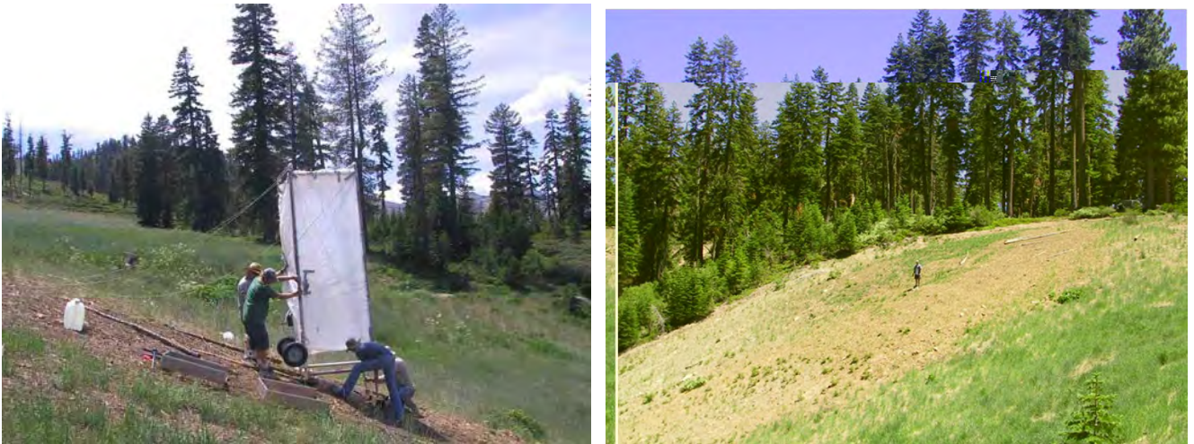
Figures 3.6 and 3.7: the photo on the left shows the rainfall simulator being set up on a ski run in the Squaw Creek watershed. The photo on the right shows a distant view of that same slope. The well vegetated area produced similar amounts of runoff and sediment yield as a bare area while the areas on both sides of the person in the photo produced no runoff in simulated rainfall events of 2.4 inches per hour. Note that those areas, which are test plots, were all tilled, some with compost and some with wood chips. The approach on these test plots was to attempt to primarily restore hydrologic function and nutrient cycling. The relatively unvegetated area in front of the person absorbed over 5 inches of rainfall with no runoff. These results indicate that control of erosion is not primarily a plant function.
