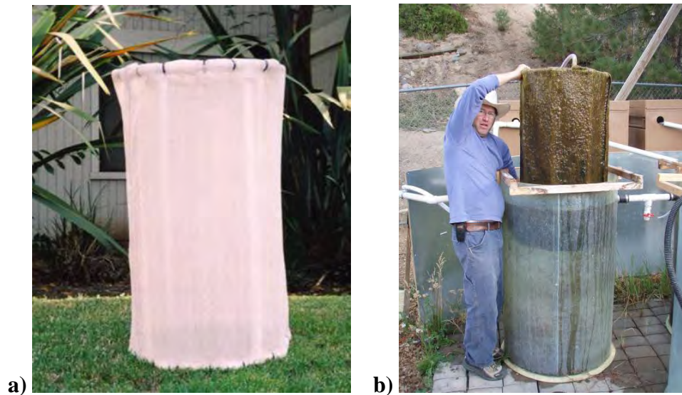
Figure 5. Periphyton substrate screen a) prior to first deployment b) with typical periphyton biofilm before harvesting.
