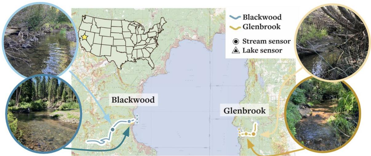
**Figure 12.** Map of stream monitoring locations at Blackwood and Glenbrook creeks. The stream is highlighted in blue for Blackwood or gold for Glenbrook and sensor positions are noted with circles for in-stream miniDOTs and HOBO conductivity loggers. Upper photos depict the upper stream reaches and lower photos depict the downstream or lower reach location.
