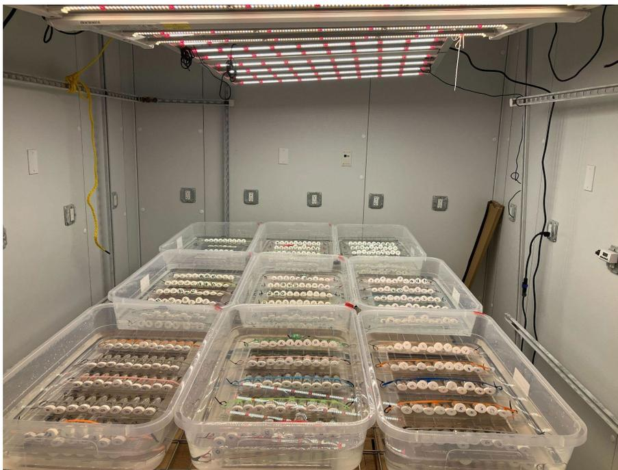
**Figure 26.** Replicate sediment and algal incubations in water baths in a temperature-controlled cold room and set under light conditions to mimic those in the nearshore zone of Lake Tahoe.
